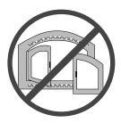
The door(s) must be closed and latched during operation. Open the door(s) only when reloading the fireplace or conducting maintenance. This prevents smoke, embers from entering the room.
